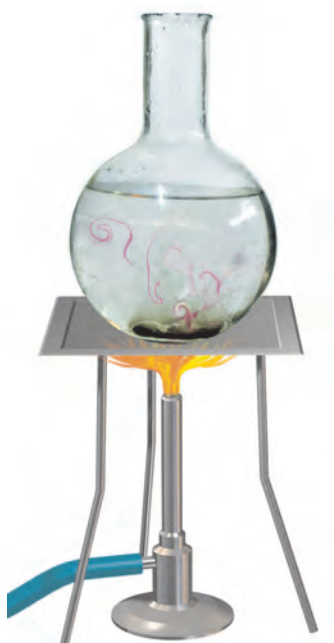
Fig. 3.9 Convection of heat in water
