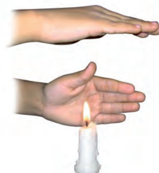
Fig. 3.10 Transfer of heat by convection in air
